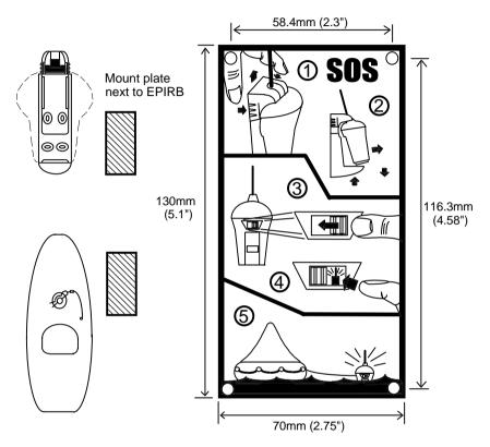
The instruction plate should be mounted next to the EPIRB so that it is easily visible in an emergency. Use the four self-tapping screws supplied to mount the plate. Mounting dimensions are shown in the diagram above, or you can use the plate itself at a drilling guide for the screws.
