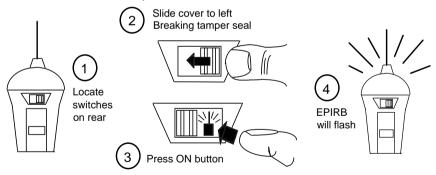
Once activated the Precision 406 <u>must</u> have its antenna near upright and it must have a clear view of the sky for proper operation. Lying it on its side or placing it next to a metal wall will impair its range and may fail to alert the rescue services. Avoid handling the antenna, as this will also impair performance.
