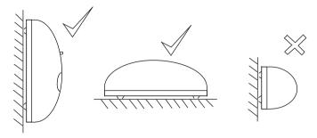
If you have a float-free Precision 406 it is critical that you choose a position where the released EPIRB will **not get trapped by overhangs, rigging, antennas** etc, should the vessel ever sink. An expanse of flat surface is required to allow the enclosure lid to eject. Use the list below to choose a suitable mounting position:
